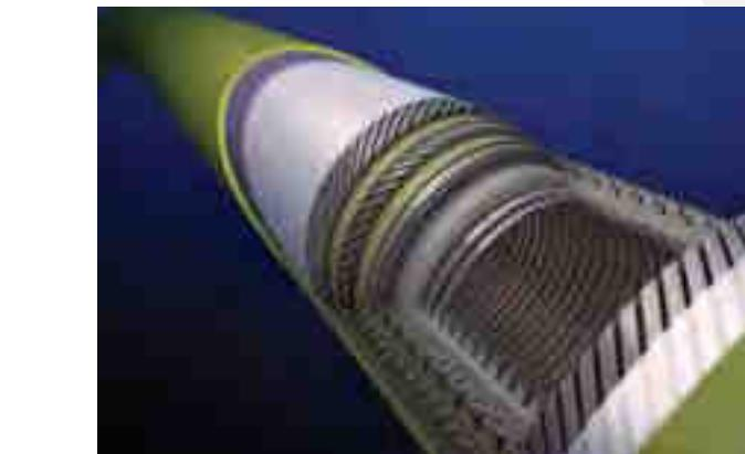
CTS flexidrain tubes are available from 3-inch to 8-inch internal diameter. It consist of an interlocking metallic carcass, inside a barrier layer. This combination of layers allows the flexidrain to be installed in a repetitive lay pattern, which ensures the safe operation of the tank roof. All tank drain flexible lay patterns are custom engineered for each specific tank.
