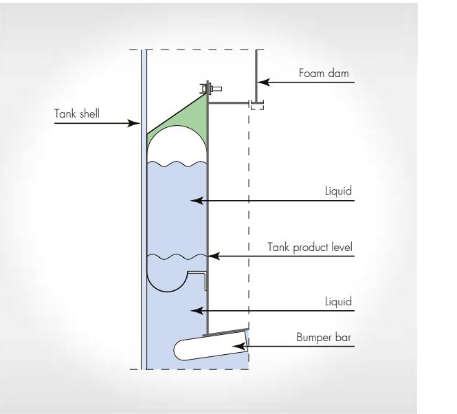
The CTS6 liquid filled primary seal consists of a wear resistant ribbed envelope containing a liquid filled tube. The inside tube can be filled with any hydrocarbon or water, subject to requirements. The flexibility of the tube and the ribbed surface of the envelope will ensure an excellent long term vapour tightness.
