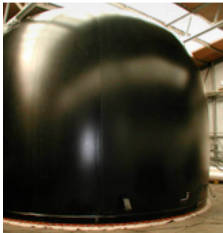
Vapour bladder during factory test.
